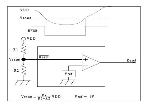
Figure 6-10 Architecture of Power-on reset circuit
