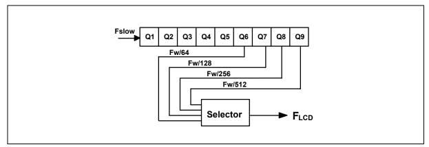
Figure 6-15 LCD alternating frequency (FLCD) circuit diagram
