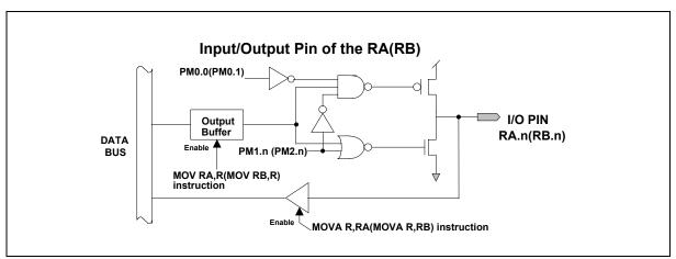
Figure 6-11 Architecture of RA (RB) Input/Output Pins
