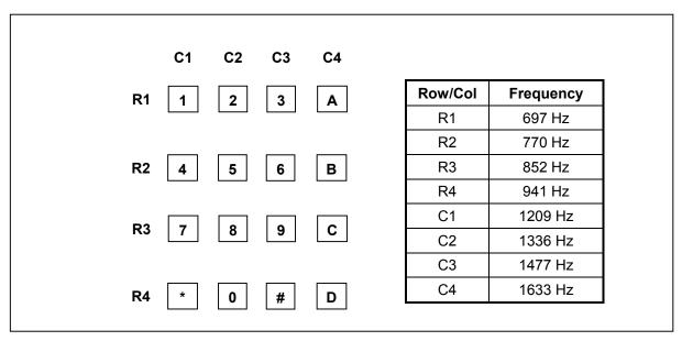
Figure 6-14 The relation between the touch tone keypad and the frequency
