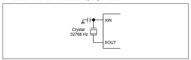
Figure 6-3 System Clock Oscillator Configuration
