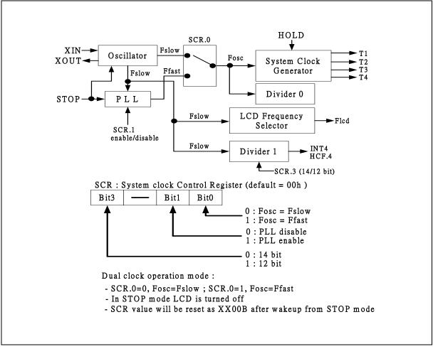
Figure 6-4 Organization of the dual-clock operation mode
