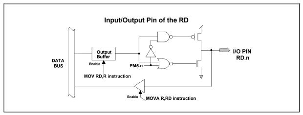
Figure 6-12 Architecture of RD Input/Output pins
