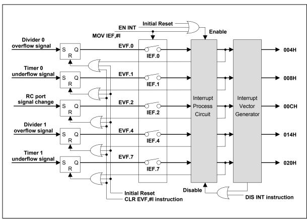
Figure 6-8 Interrupt event control diagram
