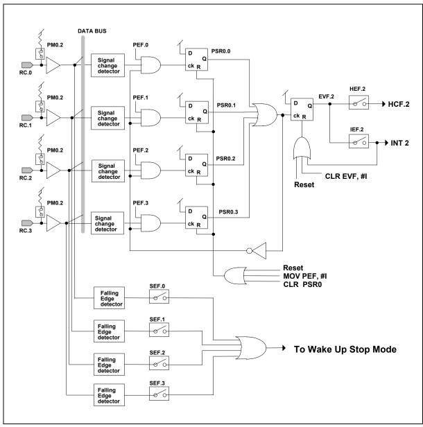
Figure 6-13 Architecture of Input Ports RC
